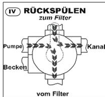
Cleaning filter medium (i.e. sand) in counter flow (reversed flow direction in filter)
