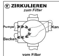
Circulating the medium without Filter (Filter is bypassed)
