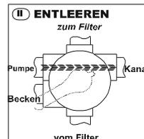
Draining of the pool with the pump
