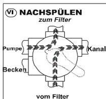
Cleaning filter medium (i.e. sand) after backwash cycle
